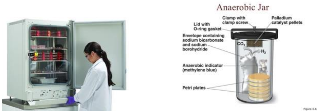
Figure 5.8. Left: Constant temperature incubator. Right: an anaerobic jar system used for excluding oxygen from cultures during incubation.
